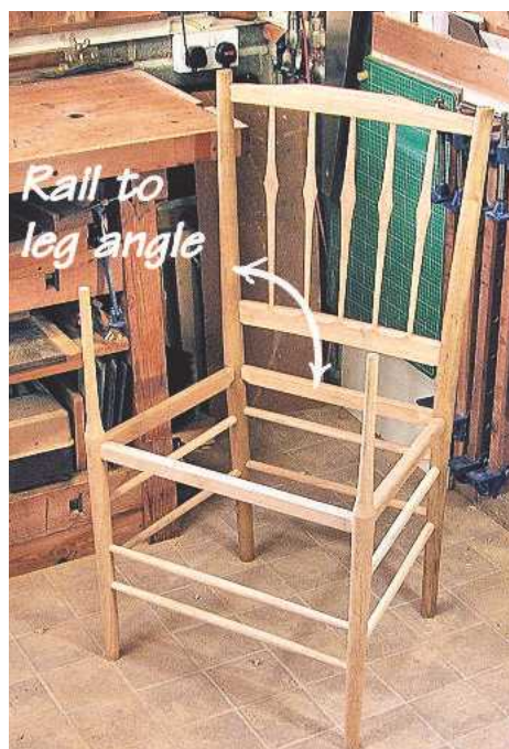
▲ Pic. 1 At this stage I could set about drilling the mortise holes for the arms
